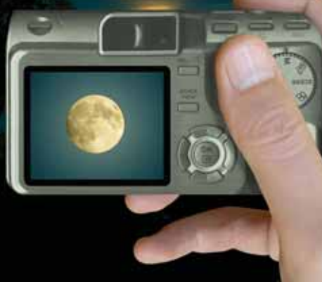
Live focusing lets you focus on an enlarged portion of the image that falls on the camera's CCD sensor. Nikolai Sorokin/Dreamstime.com
